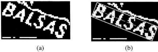
Fig. 7. (a) Label of ' BALSAS ' river is touching the line of the river at the first letter 'S'; (b) Starting with a line following the label angle, a dynamic rectangle is built
