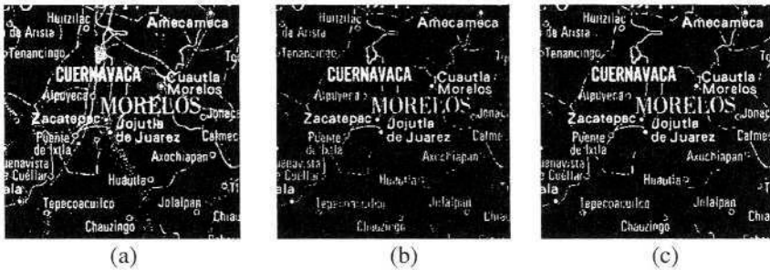
Fig. 2. (a) Binary image of Figure 1b (a high-value threshold); (b) Binary image of Figure 1b (a low-value threshold); (c) Binary image of Figure 1b (global dynamic thresholding [5])
